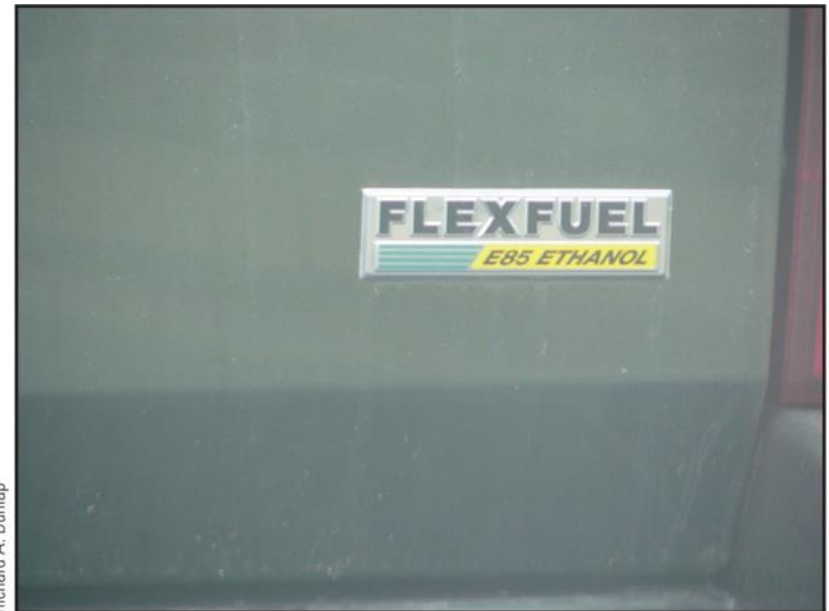
Figure 16.4: Nameplate on vehicle designed to run on gasoline with up to 85% ethanol (E85).
